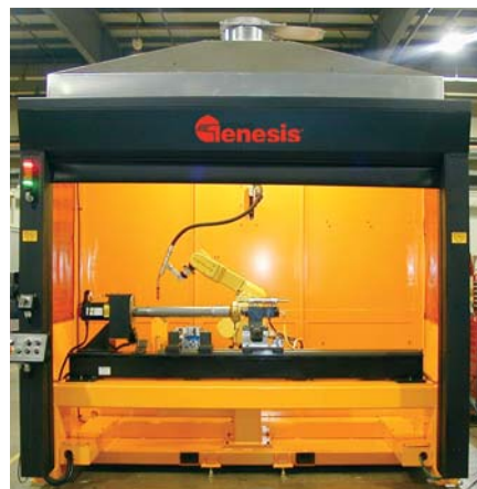
Our Compact Robot Zone (CRZ) FT is a low cost solution for welding smaller parts. The CRZ-FT can have one or two weld stations or be slightly customized like this one.
