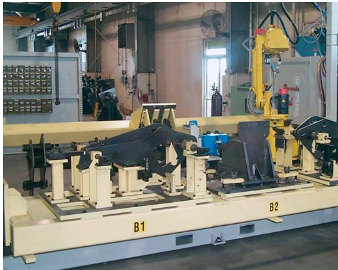
Here's a Versa 2L with the robot on a transporter to provide a greater work envelope. The Versa 2L has two weld stations and is highly adaptable to your production needs. In this example three fixture stations hold parts for welding.
