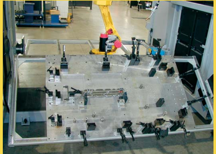
Our most popular system for Contract Manufacturers – this Versa 2L shows a weld fixture mounted on our quick-change picture frame fixture receiver. The right system if you need to run many different parts. Rentals available.
