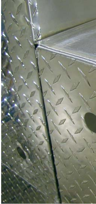
Outside corner weld (.063) on aluminum diamond deck tool box.
