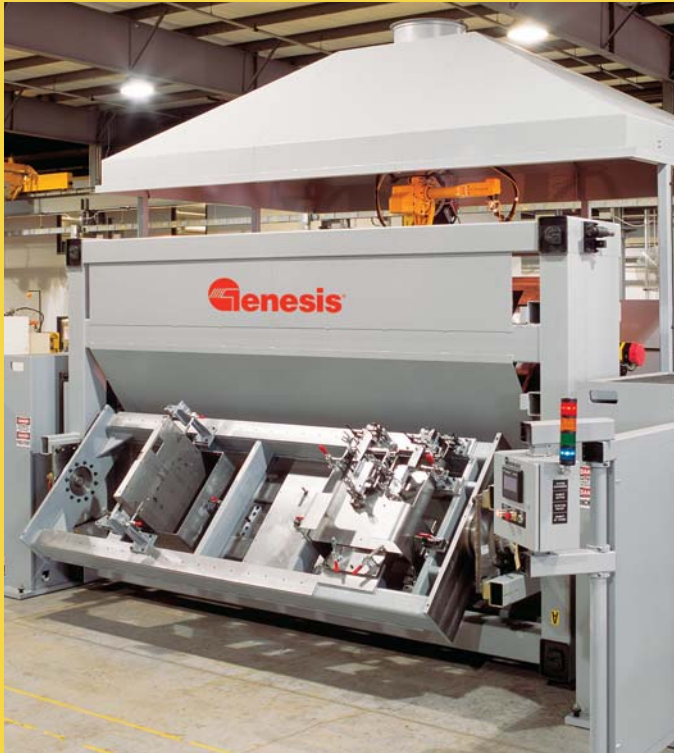
Higher production parts? The Versa 4M with 60" diameter weld fixtures mounted in each station handles heavy loads with ease and has single-point fixture loading.
