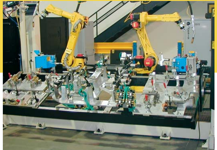
Another great example of the Versa 2L – this one with dual robots – allows each weld station to be set up with seven different fixtures and parts to weld.
