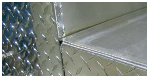
Outside corner weld (.063) on aluminum diamond deck tool box.
