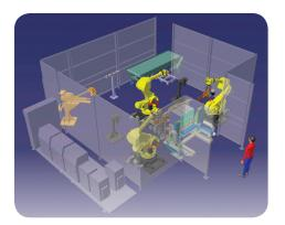
Delmia V5 allows precision robot placement to maximize robot reach with 3-D verification of all potential obstacles.
