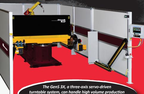
parts that require repositioning during the weld cycle.
